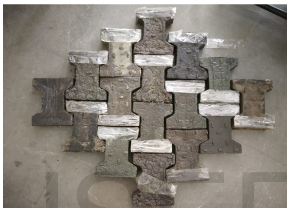
Fig. 3. Interlocking arrangement of plastic paver block.
